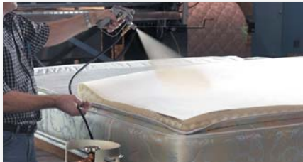
With 3M™ Foam Fast Cylinder 74 Spray Adhesive a fast light coat bonds quilted fabric to solid core mattress. High coverage reduces applied cost. Foam-tearing strength prevents cover spin.
