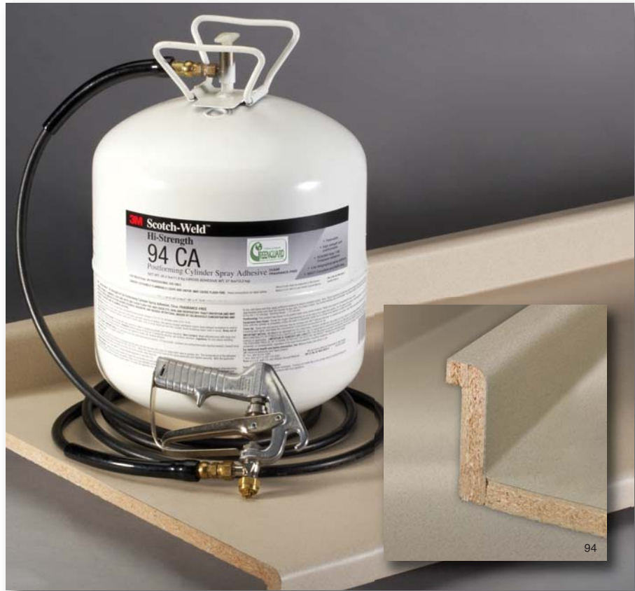
For HPL countertop assembly, 3M™ Scotch-Weld™ Cylinder Spray Adhesive 94 CA dries quickly to reach postformable strength in 1-5 minutes. 1-15 minute open time provides flexibility in assembly speed. Formulated specifically with low telegraphing for thin veneers and glossy laminates.
