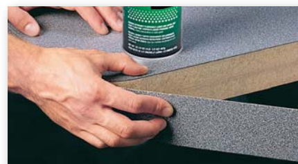
150 3M™ Hi-Strength 90 Spray Adhesive typically bonds edge banding in 60 seconds compared to 15-20 minutes for many typical bulk contact adhesives. Strength increases to an ultimate 230 psi in shear and 25 piw in peel.
