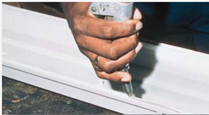
To prevent moisture penetration, a pressure flow gun applies 3M™ Scotch-Weld™ Rubber and Gasket Adhesive to bond a rubber gasket into a commercial light fixture cover.
