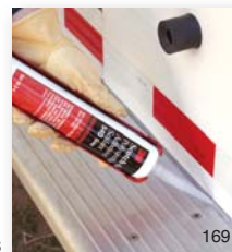
For gaps and seams outside and inside of a trailer, 3M™ Scotch-Seal™ Sealant 540 stays flexible and secure at -40° to 194°F (-40° to 90°C) compensating for thermal expansion/contraction even between dissimilar surfaces.
