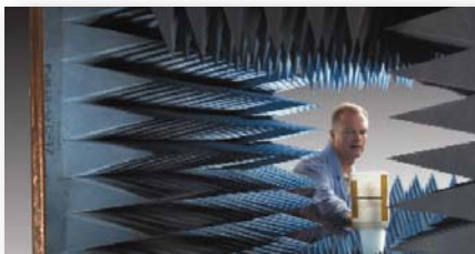
With heavy web spray and low soak-in, 3M™ Scotch-Weld™ HoldFast 70 Cylinder Spray Adhesive attaches noise abatement foam to the plywood walls of an anechoic chamber.
