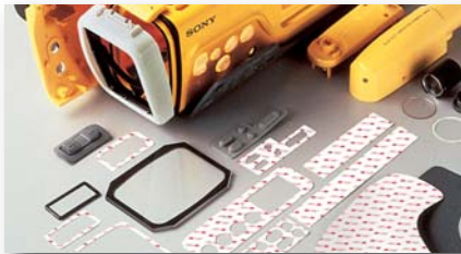
For assembly efficiency, die-cut pieces of 3M™ VHB™ Tapes bond components in a water-resistant video camera case. The foam conforms to help seal the unit. 180
