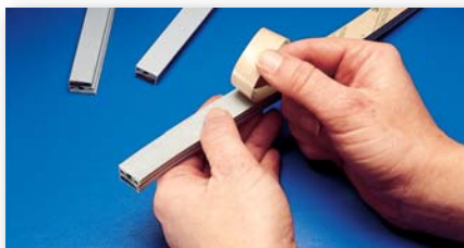
For bonding flexible vinyl in such applications as door gaskets, 3M™ Adhesive Transfer Tape F9465PC resists the effect of plasticizers that tend to migrate from the vinyl.
