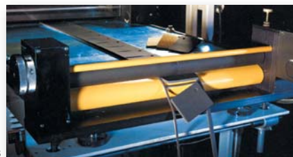
3M™ Adhesive Transfer Tapes provide conformability in a variety of foam laminating applications. The acrylic adhesive also provides high shear strength and good environmental aging properties.
